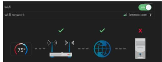
A graphical representation of the home network showing the connection status from the High Definition Display to the Smart Hub to the Internet to the Lennox server.
